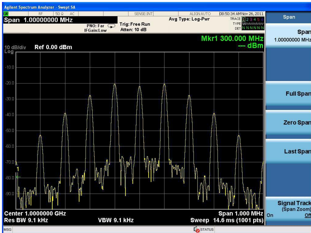
Figure 3-5 Test result of the PM modulation signal
