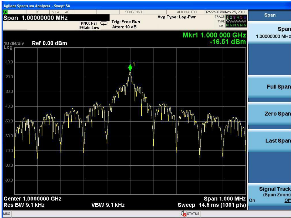
Figure 3-7 Test result of the ASK modulation signal
