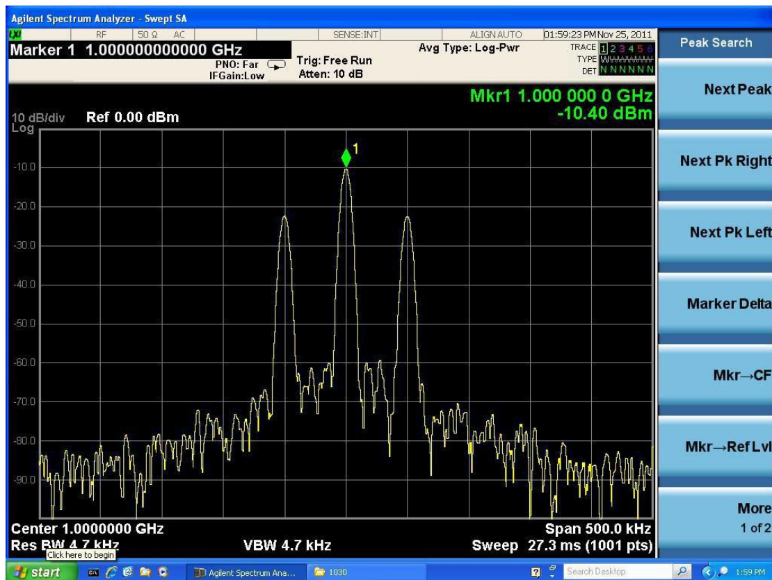
Figure 3-4 Test result of the AM modulation signal
