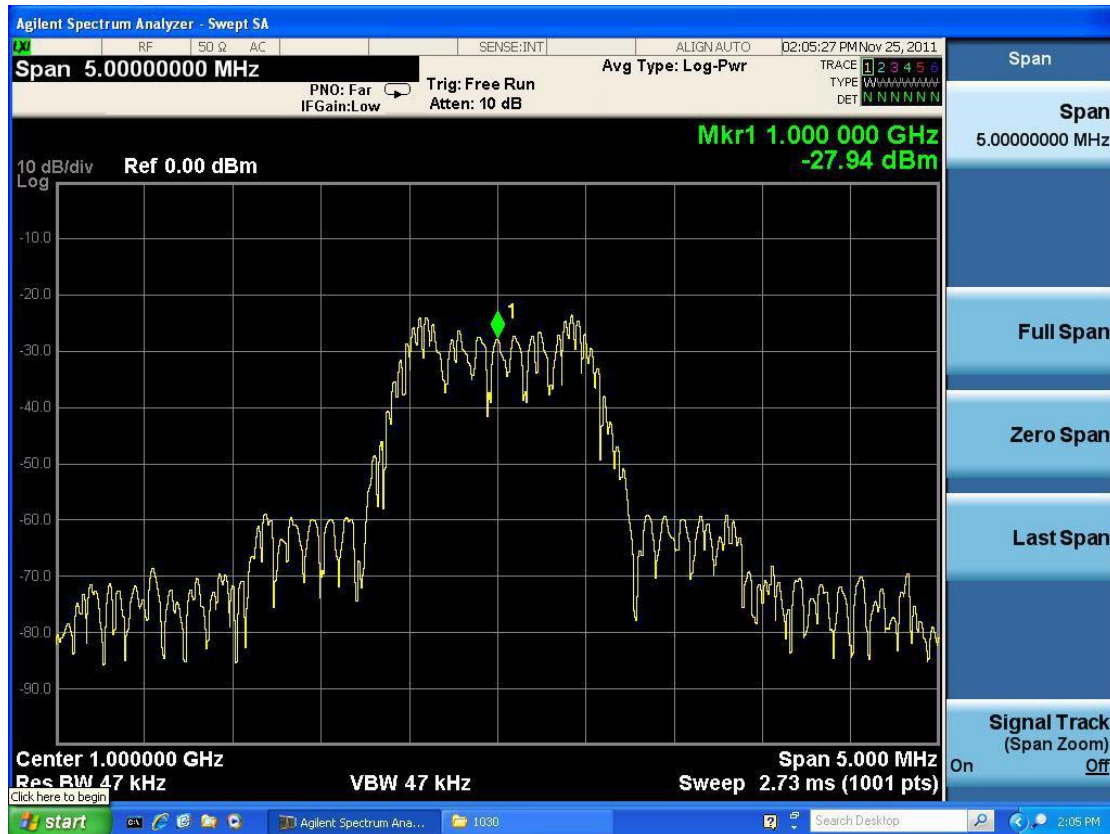
Figure 3-5 Test result of the FM modulation signal
