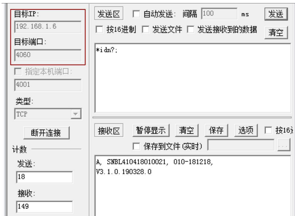
Figure 4-3 Read and write commands via LAN
