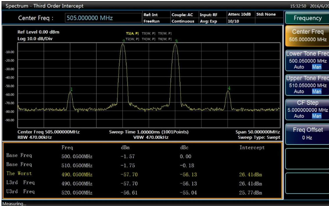
Fig. 4.79 Results of Three-order Intermodulation Measurement
