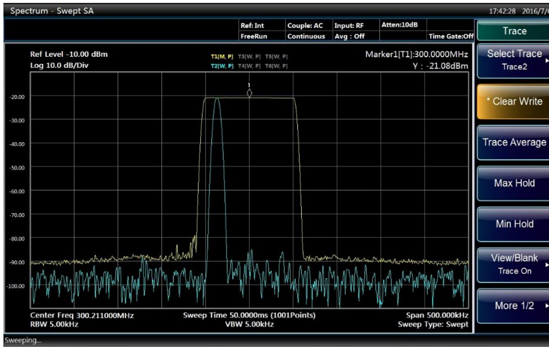
Fig. 4.37 Signal drift observation by the max hold
