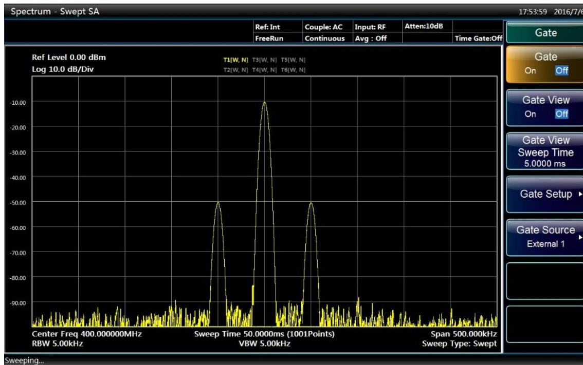
Fig. 4.60 Observed FM signal spectrum without the Gate
