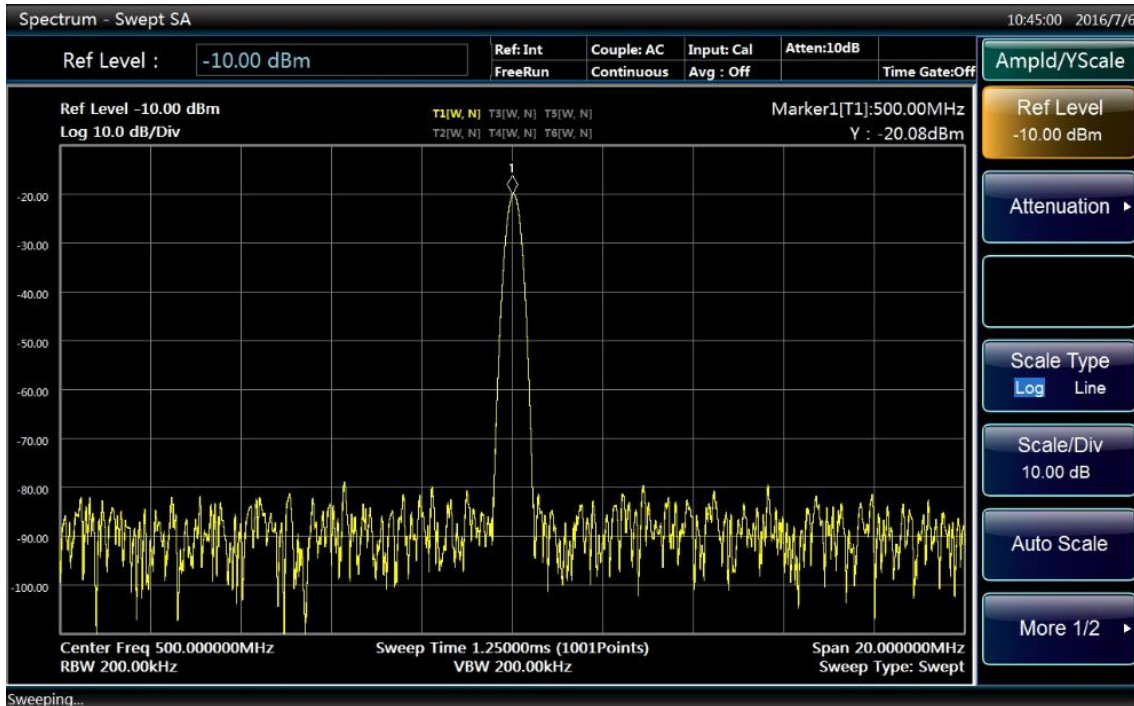
Fig. 3.18 Calibration signal spectrum after optimizing settings
