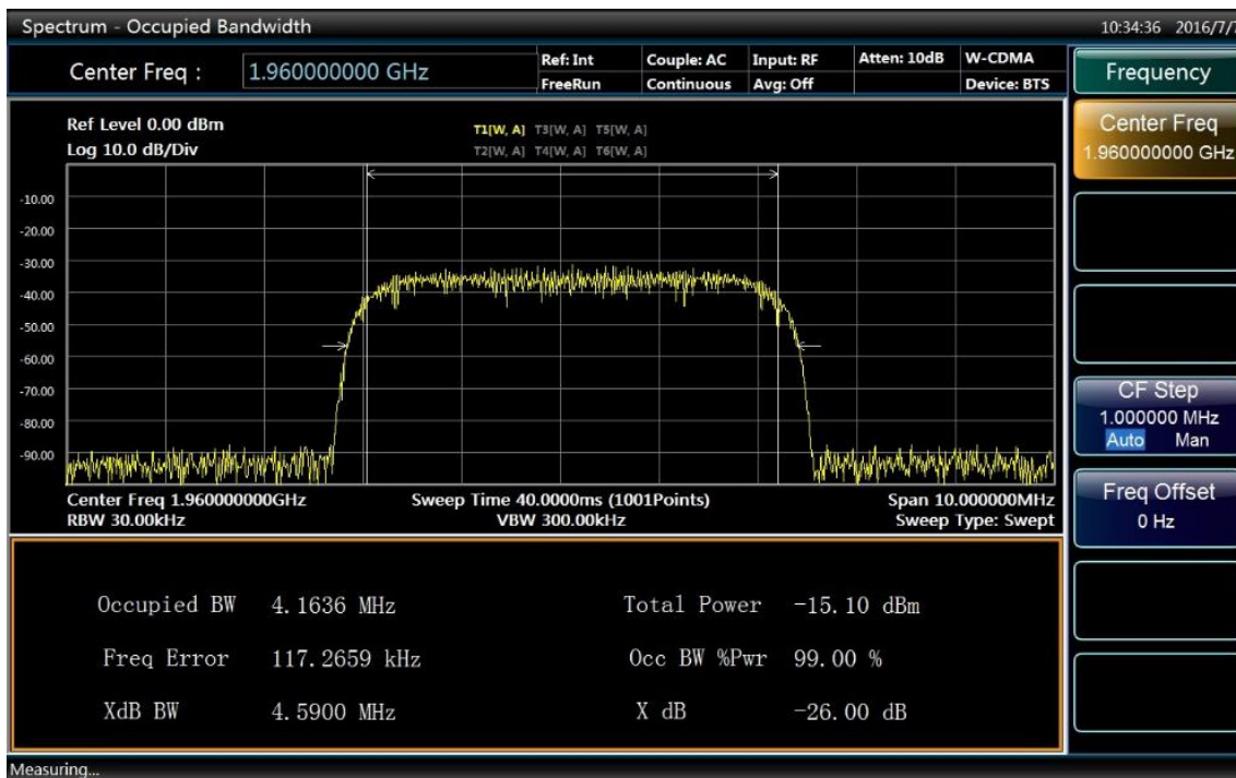
Fig. 4.64 Results of occupied bandwidth measurements
