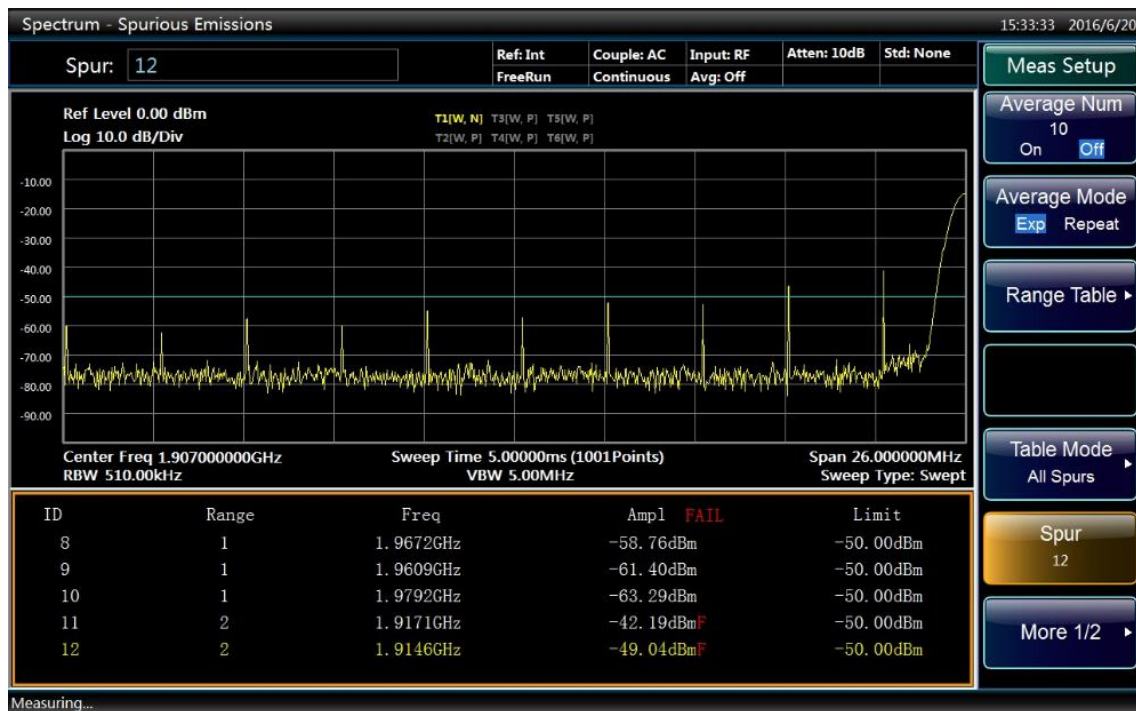
Fig. 4.81 Results of Spurious Emission Measurement
