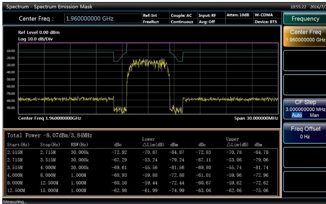
Fig. 4.83 Results of Spectrum Emission Mask Measurements
