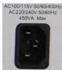
110 V/220 V self-adaptive AC power module
