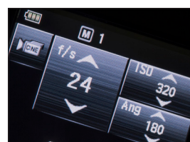
The world's first meter to offer HD/CINE and CINE mode with features such as: frame rate, shutter angle, lux, foot-candle, cd/m2 and foot-lambert.
