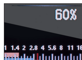
Measure ambient and flash output simultaneously. Displays ambient/flash ratio in two separate ways: on a graphic color bar, as a percentage of flash. In addition, total exposure is shown in f/stop.
