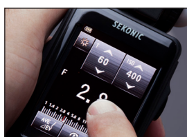
Pressure sensitive 2.7" large color LCD Screen with tap or scroll interface. Adjustable color brightness for fast, more intuitive, better interactive control.
