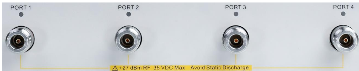
Figure 5-6 Front panel RF connectors (4-port VNA)
