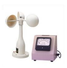
Install the 3-cup anemometer outdoor. Connenting the sonsor and the indicator with a cable, instantaneous wind speed can be monitored indoor. Self generated power.
