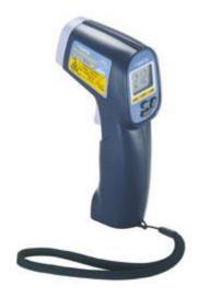
This IR meter with a wide measuring range of -40 to 450°C, is ideal for various applications. Distance to spot ratio is 10:1. Selectable emissivity of 0.95, 0.90 and 0.85 is usable for accurate measurement.
