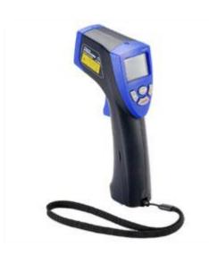
Measuring range is -40 to 500°C. This model is ideal for various applications; 10:1 Distance to spot ratio and adjustable emissivity between 0.30 and 1.00 in 0.01. The laser marker can instantly identify the target.
