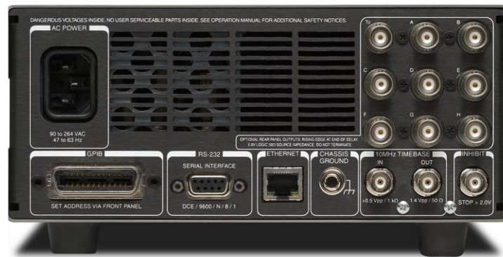
DG645 rear panel with Opt. 01 outputs
