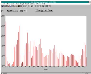
**Histogram mode** displays a bar graph of partial pressure vs. mass, allowing the spectrum to easily be interpreted. This mode is often used for quick and easy vacuum analysis. The screen can be split for viewing two modes of operation simultaneously.
