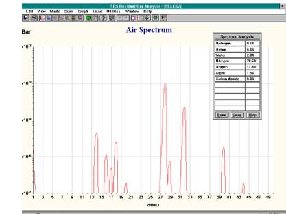
**Analysis utility** provides an approximation of the composition of gases being monitored by the RGA. Since more than one gas can contribute to a particular amu's partial pressure, the analysis mode is extremely useful in determining the make-up of complex gases. Up to 12 common gases can be selected for the analysis.
