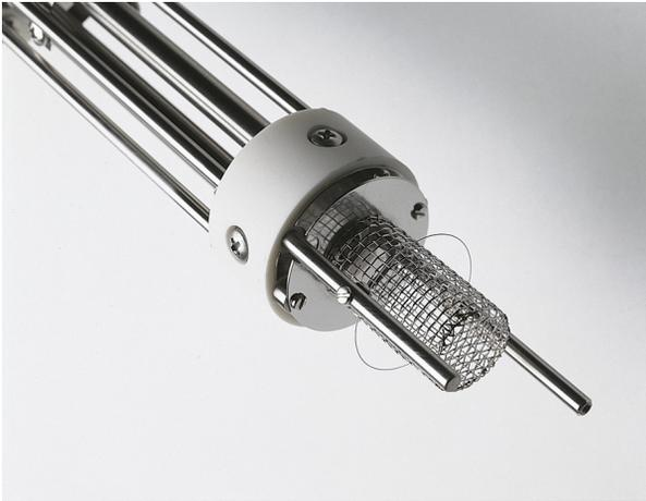
*Dual  $\text{ThO}_2/\text{Ir}$  filament*
