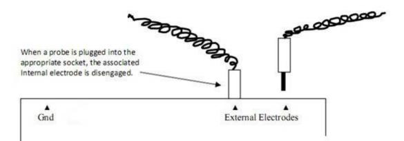
By utilizing these probes to the S2020RHR's sockets it is possible to measure Point to Point (RTT) Resistance, Surface to Ground (RTG), and Volume Resistance. Using these probes will allow compliancy with various standards including ANSI/ESDA S4.1 for Worksurface - Resistance Measurements, ANSI/ESDA S7.1 Resistive Characterization of Materials - Floor Materials.
