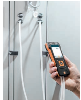
With the testo 440 dP model, which includes a differential pressure sensor, you can ensure that the filters in air conditioning systems are working properly and no contamination in the outdoor air gets indoors.
