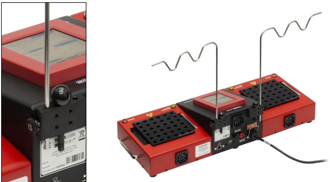
Figure 5 Install Fiber Holder(s)
