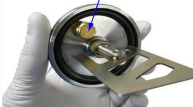
Metal filter prevent soild particals from being sucked into the vacuum pump
