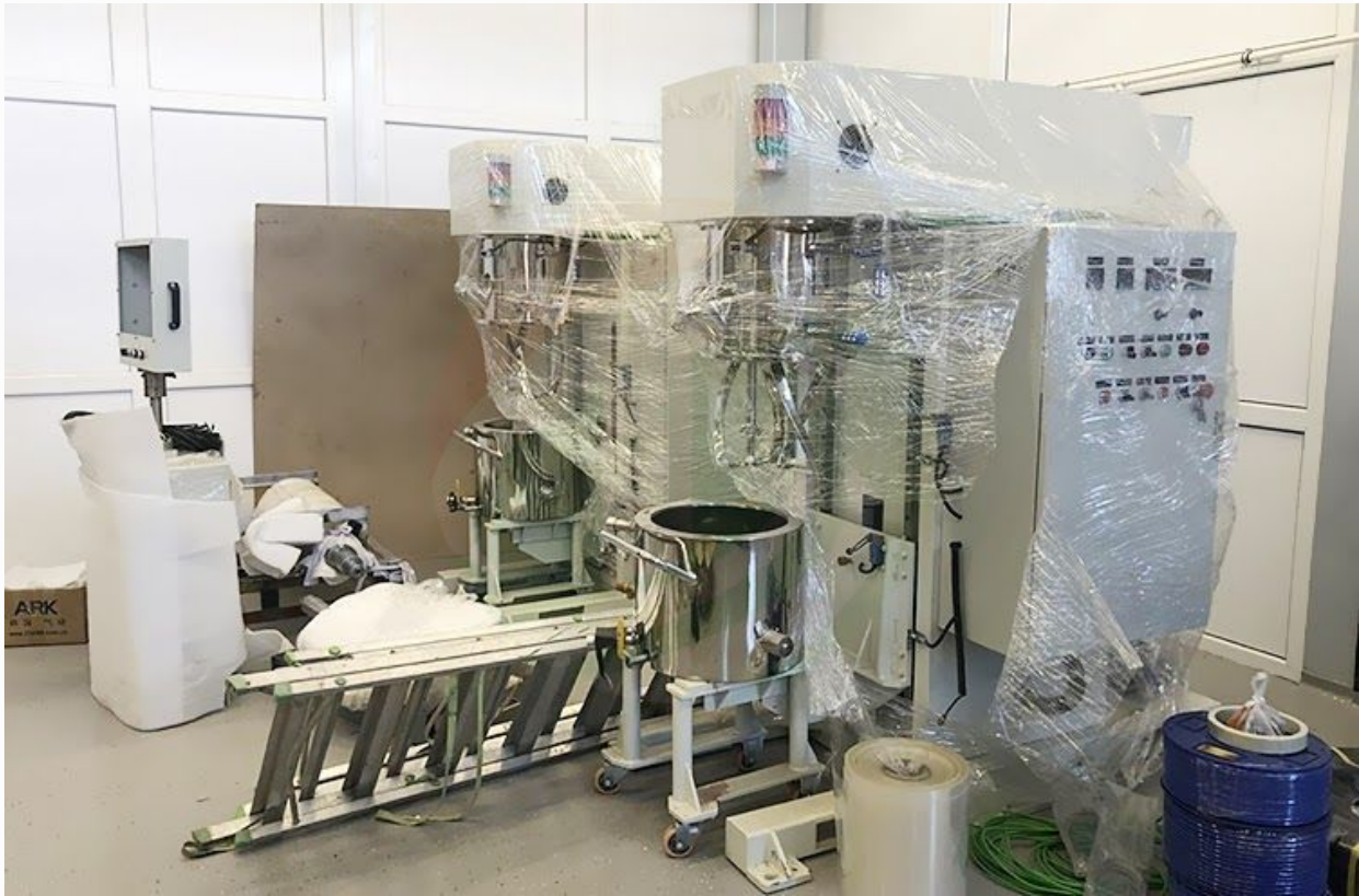
5L and 30L battery mixers used for Russian pouch cell and cylindrical cell projects
