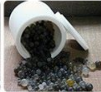
Ptfе tank and agate balls
