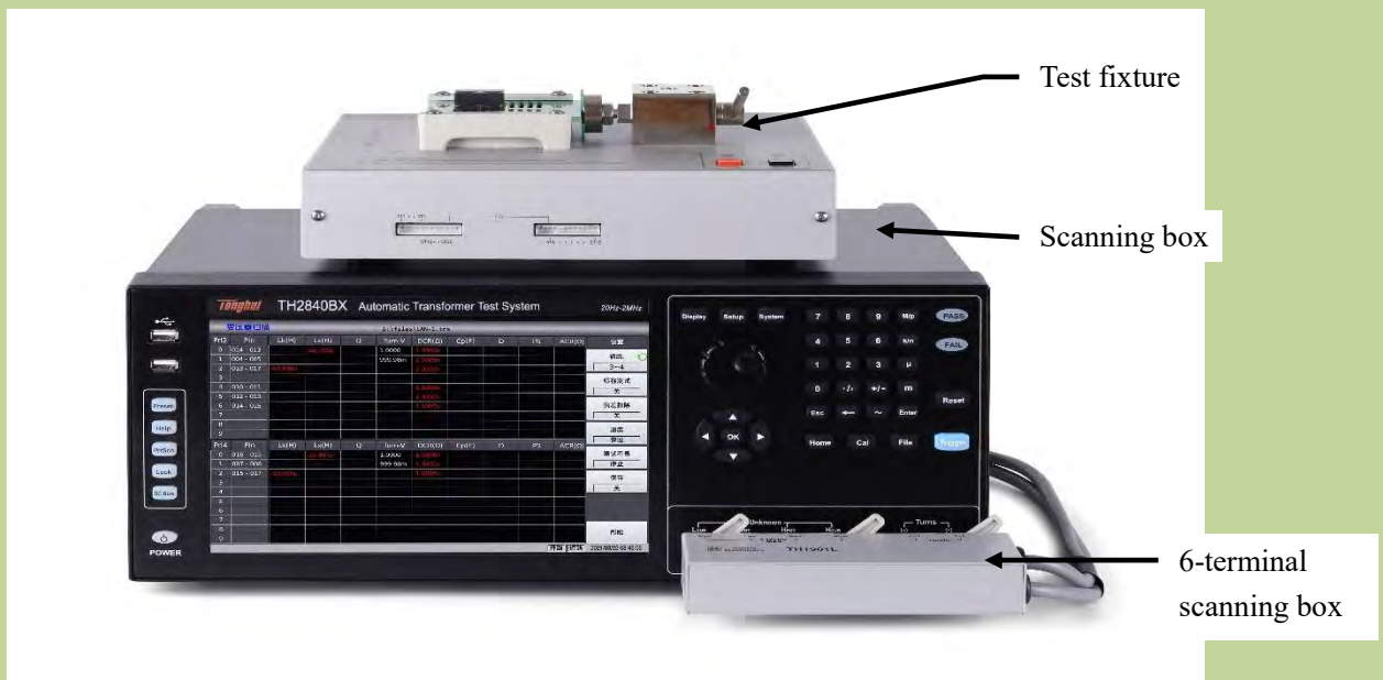
Connect the scanning test cable to TH2840X
