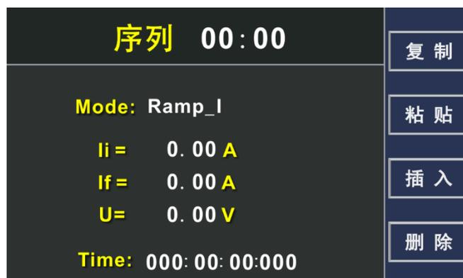
Figure 3-18 Current Slope Mode
