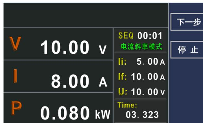
Figure 3-13 Sequence Test Single-step Run Interface
