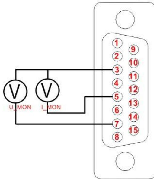
Figure 3-42 Monitor Output Voltage and Current Value
