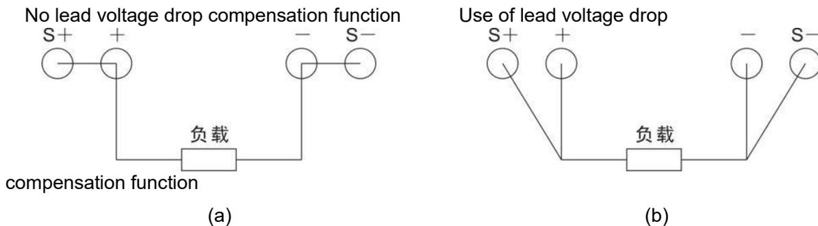
Figure 1-1 Output Wiring
