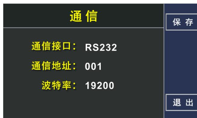
Figure 3-6 Communication Interface Setting
