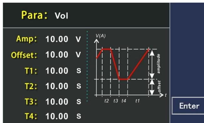
Figure 3-32 Output Trapezoidal Waveform
