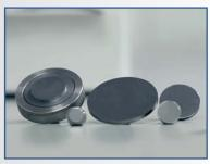
The micrometer has the option to vary pressure. A variety of pressure foot weights are available to increase the pressure on the upper anvil.
