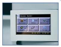
Testing is quick and easy. Parameters are software controlled and can be adapted, such as gap height, auto test mode, auto-zero and dwell time.
