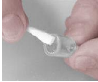
Figure 4. Cleaning Lamp Window
