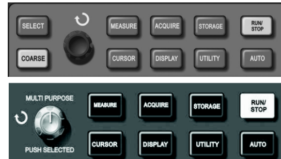
Figure 2-29 Function key (or cursor) of sampling system
