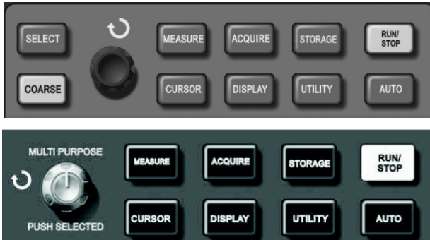
Figure 2–27 Function key (and function) of sampling
