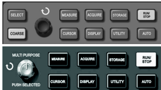
Figure 2-28 Function key (automatic measurement) of sampling system
