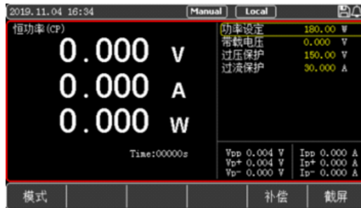
Figure 4-1-4-1 Setting Interface of CP Mode
