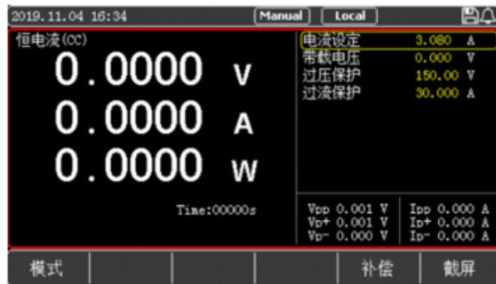
Figure 4-1-1-1 Setting Interface of CC Mode
