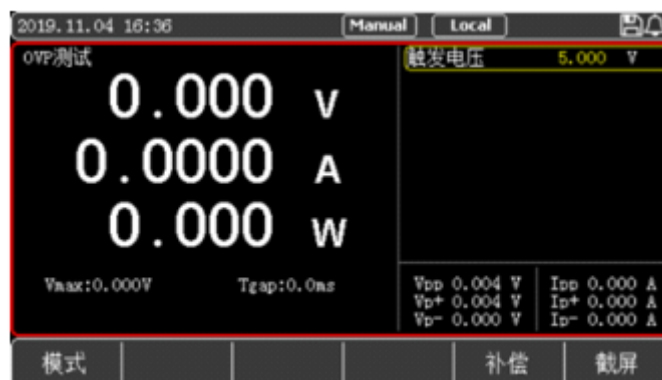
Figure 4-2-8-1 Interface of OVP Mode
