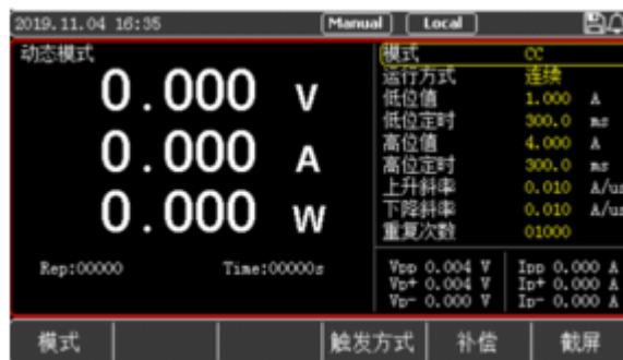
Figure 4-2-1-1 Interface of Dynamic Mode
