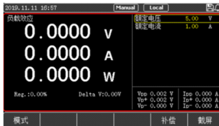
Figure 4-2-7-1 Interface of Load Effect Mode
