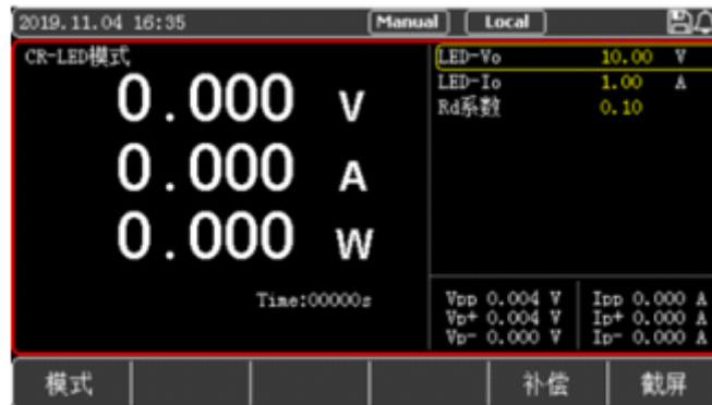
Figure 4-2-5-1 Interface of CR-LED Mode
