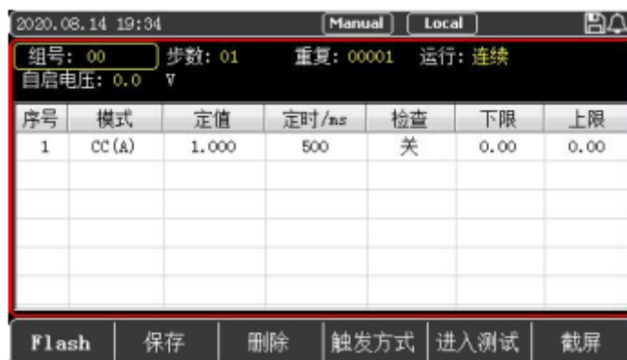
Figure 4-2-2 Setting Interface of List Mode
