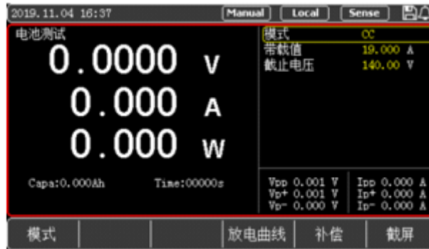
Figure 4-2-6-1 Interface of Battery Mode
