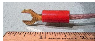
Figure 37 – “SL-48” Low Thermal Leads
