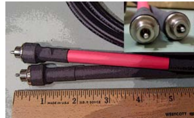
Figure 36 – “MP-5” Surface Probes
