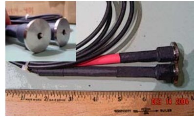
Figure 35 – “MP-4” Surface Probes
