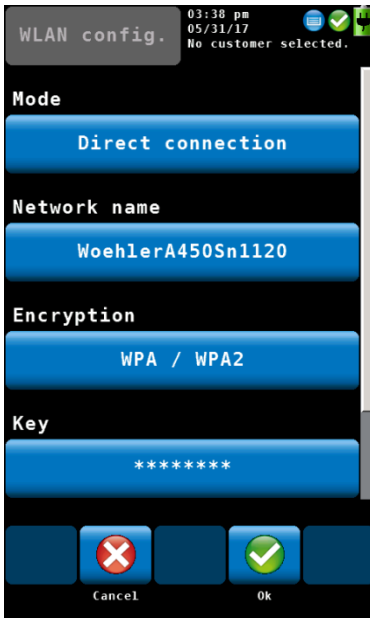
Fig. 28: WLAN configuration – Direct connection
