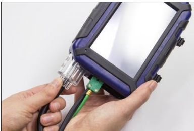
Fig. 37: Pulling the condensate trap out of the analyzer
