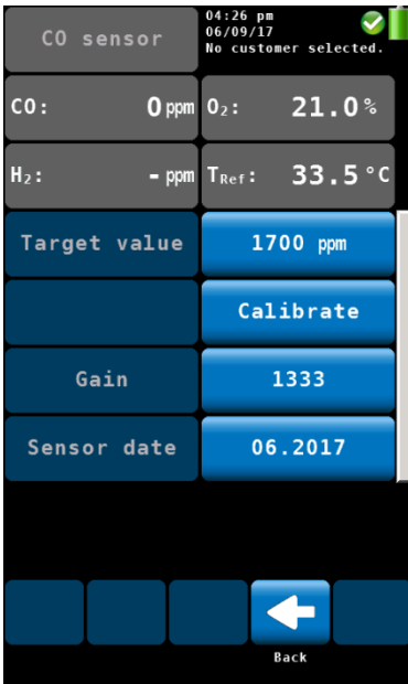
Fig. 49: Entering the calibration values in the calibration menu (only CO-sensor)
