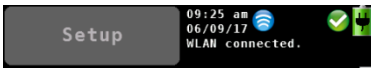
Fig. 30: „WLAN connected“ appears in the upper display, alternating with the selected customer
