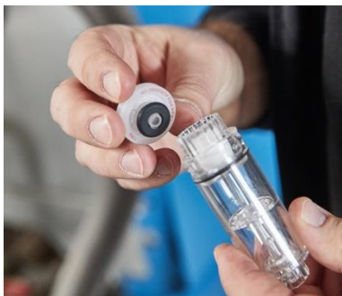
Fig. 41: Filter holder with water stop filter.
