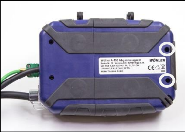
Fig. 43: Bottom of the device - Open the cover by loosening the cross-head screws .
