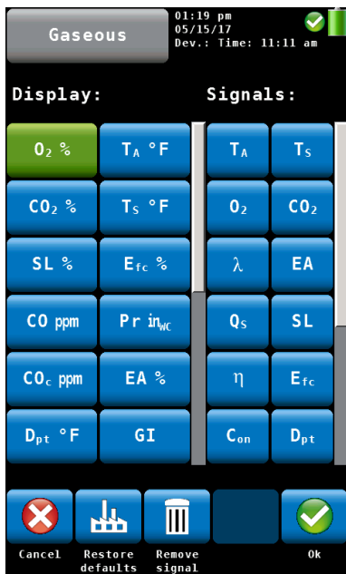
Fig. 31: Configuration of the readings segment.
