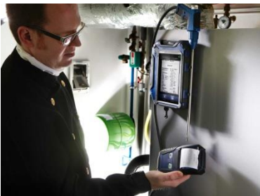
Fig. 16: Printing the readings of the Wöhler A 450 on the Thermoprinter Wöhler TD 100.
