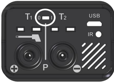
Fig. 18: Battery lock to the right: Battery activated; Battery lock to the left: Battery locked
