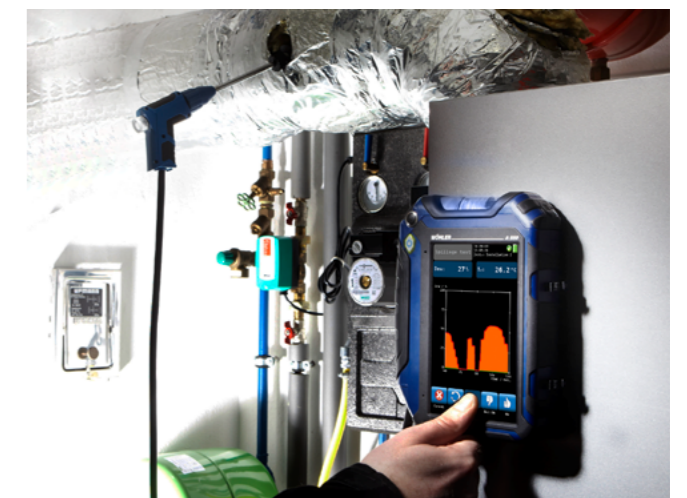
Spillage Test Optional probe available to test for back-draught conditions in the chimney.
