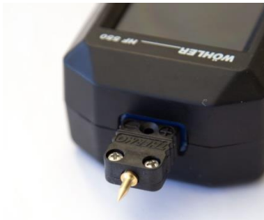
Fig. 22: Bottom of the meter with temperature probe connected.
