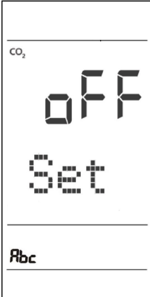
Fig. 16: ABC-Calibration (Auto Background Calibration)
