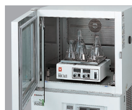
Incubator IN604W slide shaker stage (optional) and MK161 installation example
